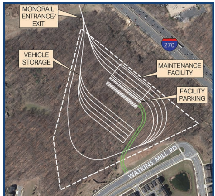
Figure 2.8 – Southern Maintenance and Storage Yard
