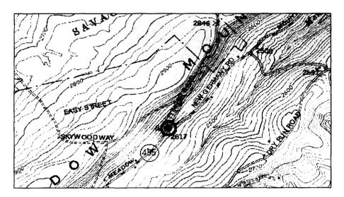
**<u>DESCRIPTION</u>**: Redesign of intersection is intended to provide a perpendicular intersection of roads with improved site distance in both directions. The project will necessitate exchange of property currently owned by the Department of Natural Resources and Garrett County. The project is intended to be a SHA/ County partnership.
