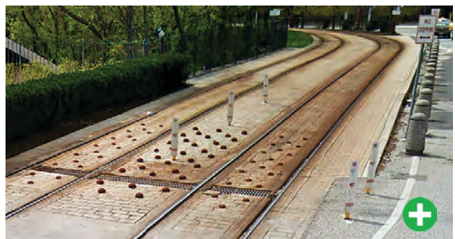
Embedded tracks are frequently found in urban streets running light rail and streetcar systems. In some places it is acceptable for all modes to share the road right-of-way, but in other areas, the use of bollards or other elements are effective to buffer the rail alignment. Source: KAI
