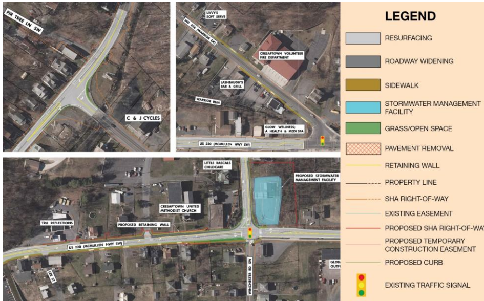
Figure 2: Proposed roadway improvements at 30 percent design completion
