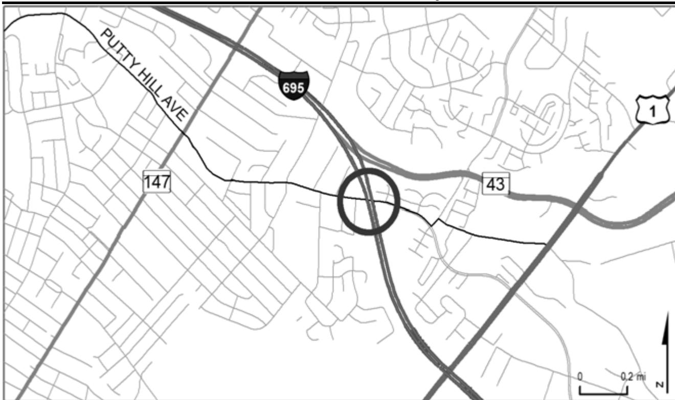
**PROJECT:** I-695, Baltimore Beltway**DESCRIPTION:** Replacement of Bridge No. 0317400 on Putty Hill Avenue over I-695.**PURPOSE & NEED SUMMARY STATEMENT:** The purpose of this project is to replace a poor rated and weight restricted bridge to keep the roadway safe and open to traffic.**STATE GOALS:** Maryland Transportation Plan (MTP) Goals/Selection Criteria:
