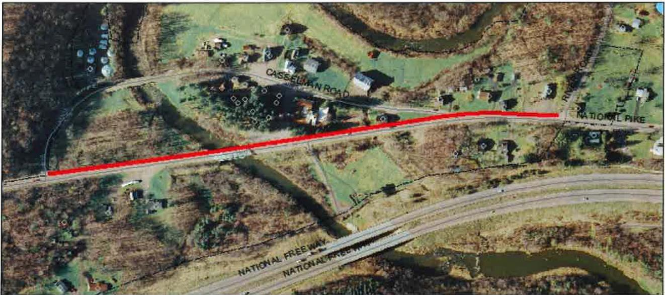
**DESCRIPTION:** The County would like to see the installation of a sidewalk along National Pike/Rt 40 between the access road for the Casselman River Bridge State Park and River Road (approximately 2,100 feet). Stormwater facilities will be incorporated into the sidewalk design to accommodate existing drainage patterns.
